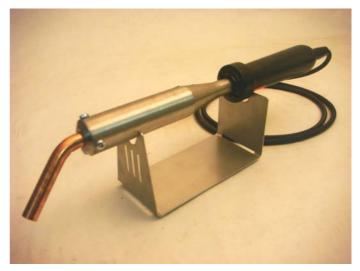
Depending on the type of alloy used, or simply for reasons of energy conservation, it is interesting to adjust the tip temperature. For exemple, to TIFFANY works the alloy Sn40Pb60 melts at 240°c can be worked with a tip at 350 ° C while for the leaded stained glass that melts at 327 ° C, a minimum of 400 ° C is necessary.
